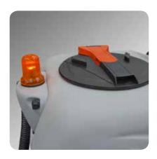
Quick lock recovery tank cap allows for fast and esy cleaning and sanification of the tank; the tilting tank together with a large size drain hose allow the complete emptying of the tank and the removal of any type of solid dirt. The antifoam device protects suction motor, as well as the electronic floating switch that stops suction when the tank is full.
